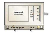
When you move the thermostat up more than 2 degrees, the system's expensive auxiliary heat will kick on.
