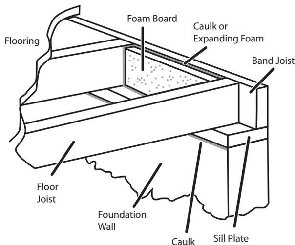
Cut 1- or 2-inch-thick foam board pieces to a rectangular size and insert between the floor joists, just above the foundation. Make sure the pieces fit snug against the joists on the left and right, and from the top of the foundation to the flooring. The edges are then sealed on all four sides with a bead of caulk or expanding foam.
